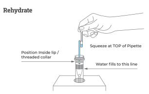
Position your filled Pipette inside the lip/ threaded collar of the Test Tube.
